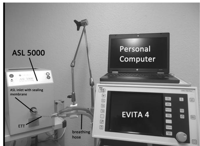
**FIGURE 1** Schematic pictogram (left) and black-and-white picture (right) showing the experimental setup with the ASL 5000 intubated with an ETT through the tight sealing membrane and connected to the EVITA 4 ventilator for measurements during spontaneous ventilation. The personal computer was linked to the ASL 5000 and collected data via the specific ASL software
