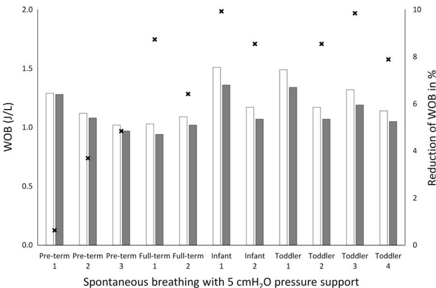
FIGURE 3 Mean work of breathing (WOB [J/L]) during spontaneous breathing with 5 cmH<sub>2</sub>O pressure support for the different lung settings. Unshortened ETT: white bar, shortened ETT: gray bar, and reduction of WOB in percent as cross
